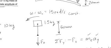
$$D = \frac{F_0 / k}{1 - (\frac{\omega_0}{\omega_n})^2} = \frac{16.875 \,\text{N}}{4905 \,\text{N/m}} = 0.00635 \,\text{m}$$
